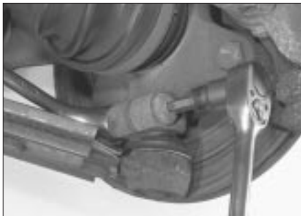
2.11a Remove the lower arm-to-spindle carrier pinch bolt and nut . . .
