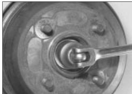
9.4 Undoing the hub bearing retaining nut
