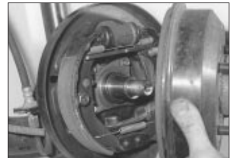
9.5 Slide off the wheel hub/brake drum unit
